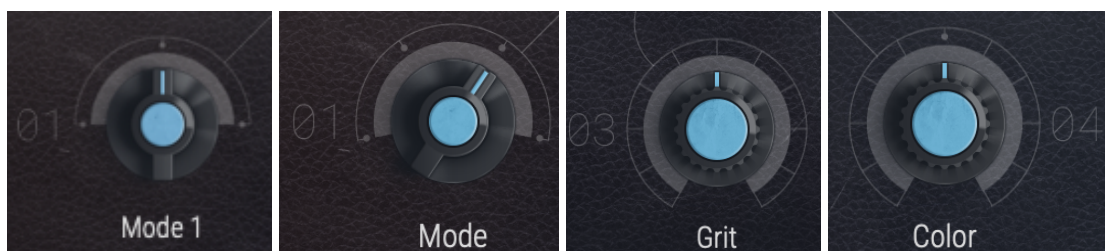
From left to right: Three-way switch, Four-way switch, Unipolar knob (zero position left), bipolar knob (zero position center)
